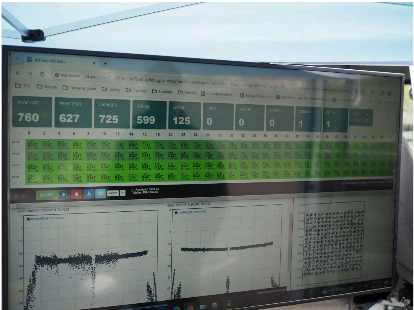
The big board in the parking lot shows status of throughput and interference, with peak throughput in this case of almost six hundred megabits per second download.
