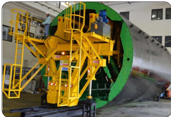
Tunnel Lining Gantry
