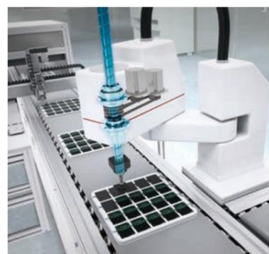
Horizontal articulated robot (SCARA robot)
