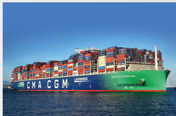
● CMA CGM SORBONNE, a CMA CGM 23,000 TEU dual-fuel LNG-powered container ship
