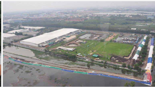
As the flood waters approached local employees protected the factories by setting up a "miracle embankment" which involved working day and night stacking up sandbags
