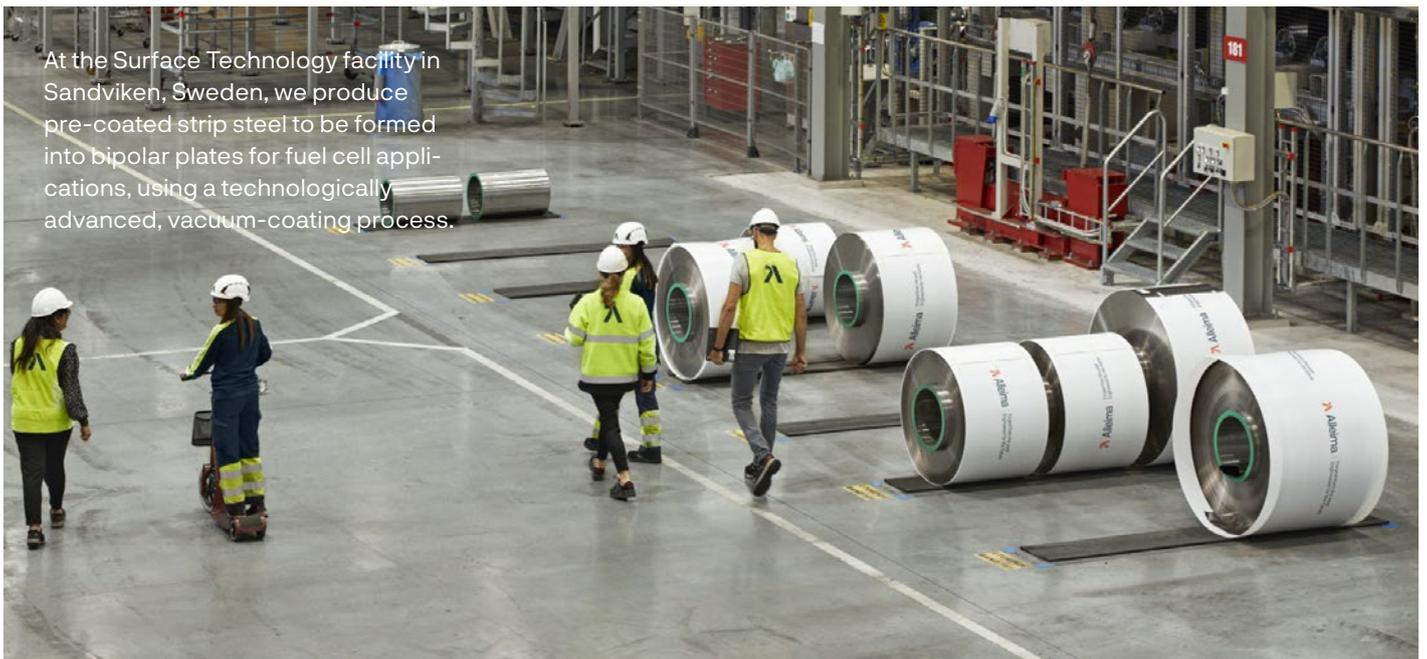
At the Surface Technology facility in Sandviken, Sweden, we produce pre-coated strip steel to be formed into bipolar plates for fuel cell applications, using a technologically advanced, vacuum-coating process.
