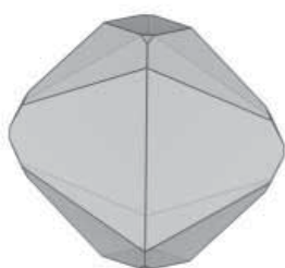
RDX crystal shape and pattern of solvent inclusion
