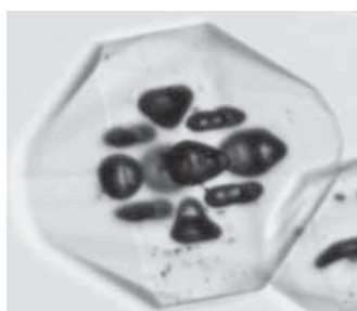
RDX crystal shape and pattern of solvent inclusion
