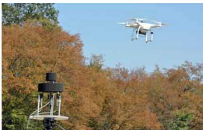
Acoustic detection of UAVs
