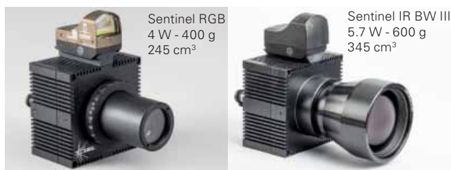
ISL's visible (left) and infrared (right) Sentinel UGS
