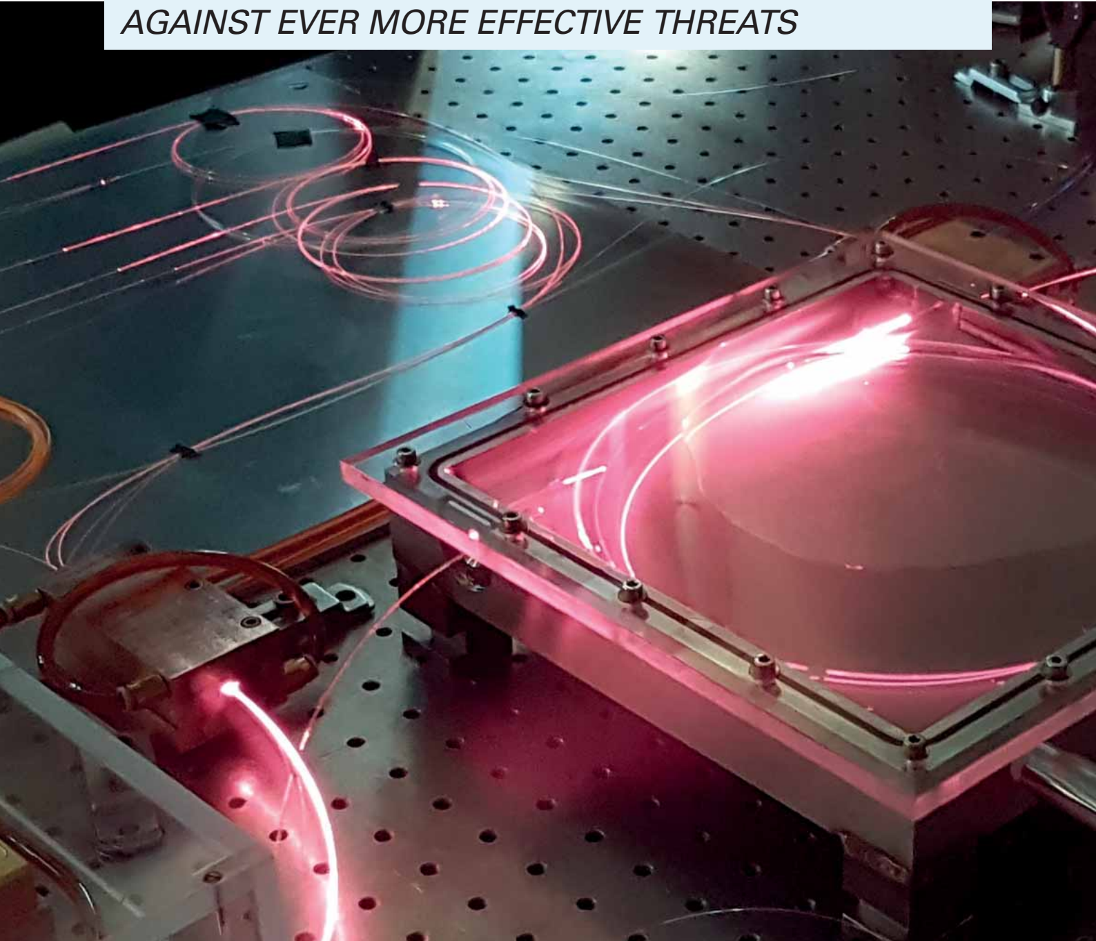
Alignment-free all-fibred laser set-up
