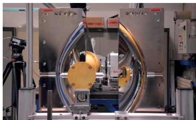
Test-bench to measure transmission and reflection of laser beams
