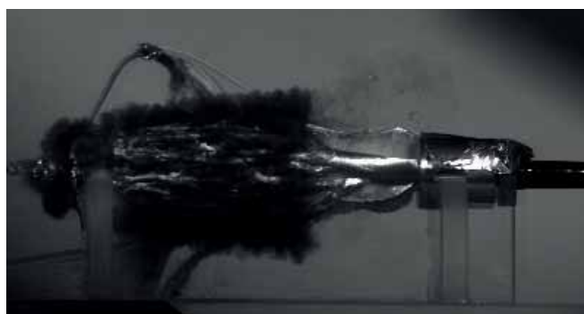
Study of the combustion to deflagration to detonation transition
