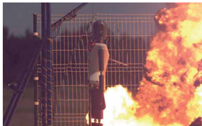
Investigating the human body vulnerability to blast waves using numerical simulation (left) and experiment (right)
