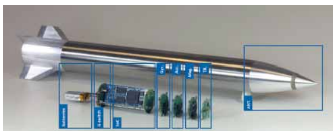
Components of an embedded navigation unit
