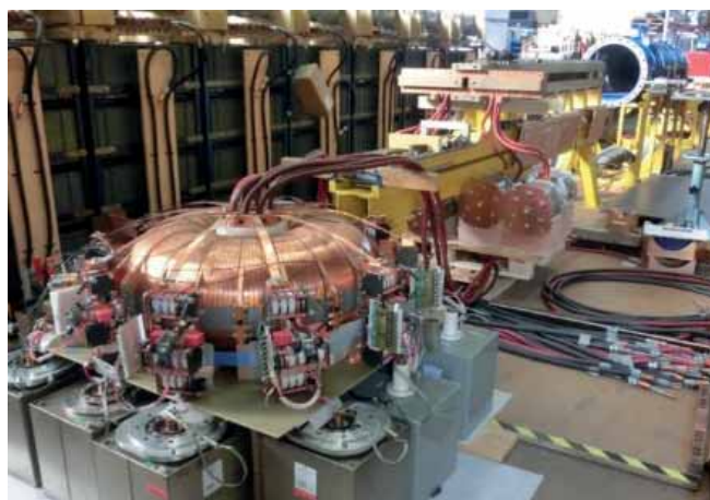
ISL's XRAM inductive pulsed power supply
