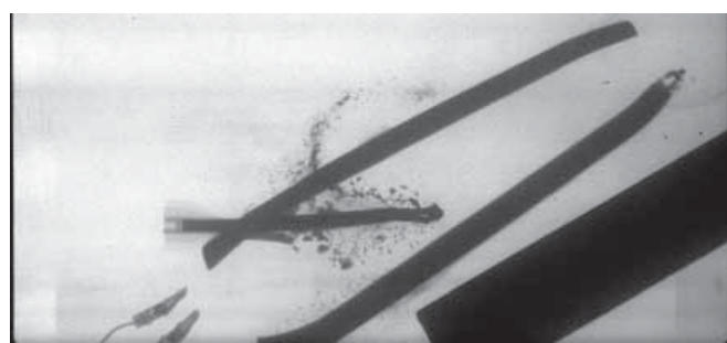
Active-ERA interacting with a long rod penetrator
